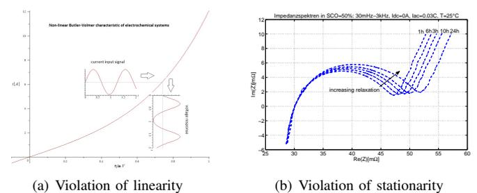
Figure 2. Error sources for valid EIS measurement
