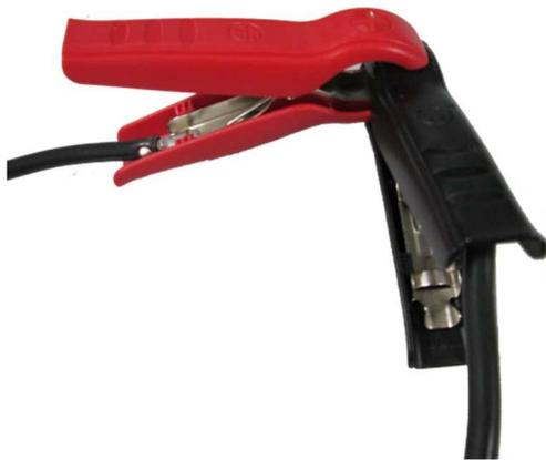
**Figure 3: Charging clips in a short circuit**
