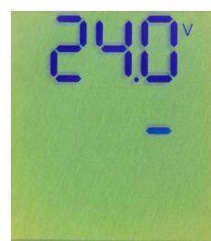
After the desired target value has been set, it can be taken over. This happens through simultaneous pressing of buttons „↓“ and „↑“ at visible "OK" indicator.
