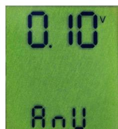
3. Selection „Analog Input 0...10V“ for the voltage target value
