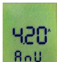
4. Selection „Analog Input 4...20mA“ for the voltage target value
