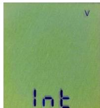
Press „ENTER“ for the input of the voltage target value.
